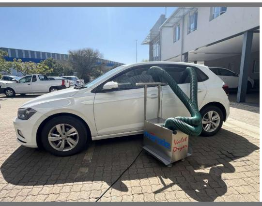
Once a vehicle has been through the valet process, time and during winter may not allow the outside ambient temperature to dry the interior of the vehicle quickly enough. For this purpose we supply a valet dryer that consists of a blower, heater and two hoses that are inserted through the car windows. This heating of the interior greatly reduces the drying period.
