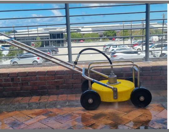
The Universal Roof and Surface Cleaner can be used with any high pressure cleaner. A good cleaning result is achieved with machines supplying 16 l/minute and higher.
